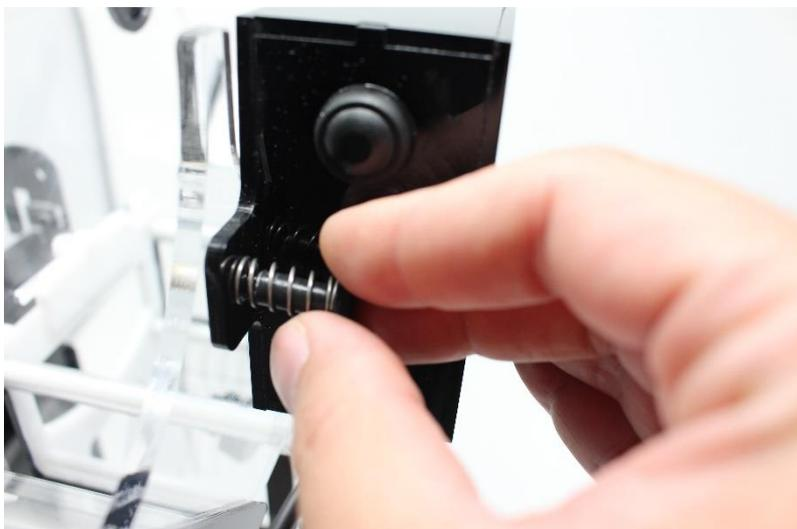
Set the long black screw with the **spring** to secure the black box with the top unit. Turn the screw clockwise and make sure the screw doesn't protrude on the other side.
