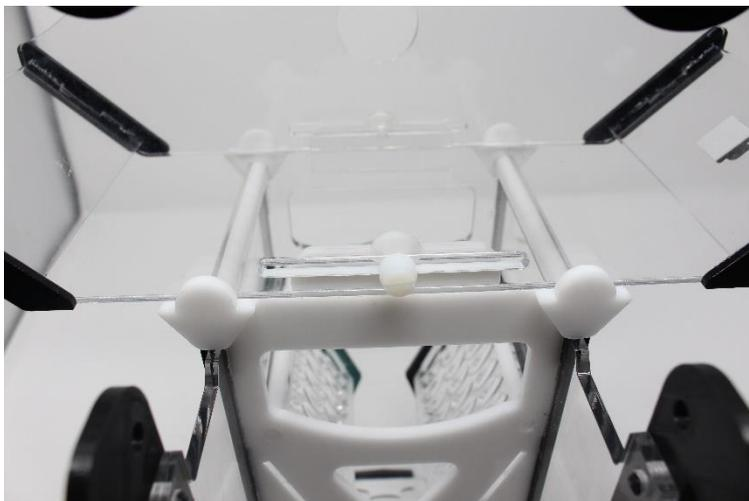
After setting the position of the top module, ensure front and back screws (back screw shown) are tight enough to restrict movement of the top module
