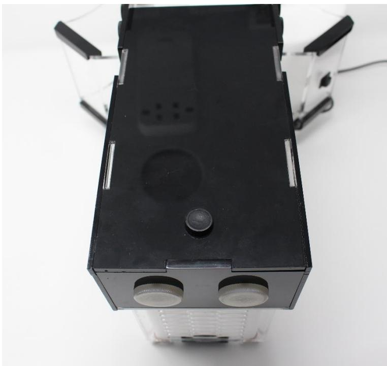
The bypass controllers are controlled by the external white discs at the bottom of the unit, as displayed.
