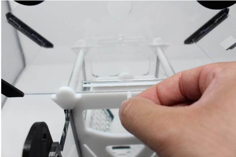
Repeat the process for the back of the unit to secure the top section to the main unit.
